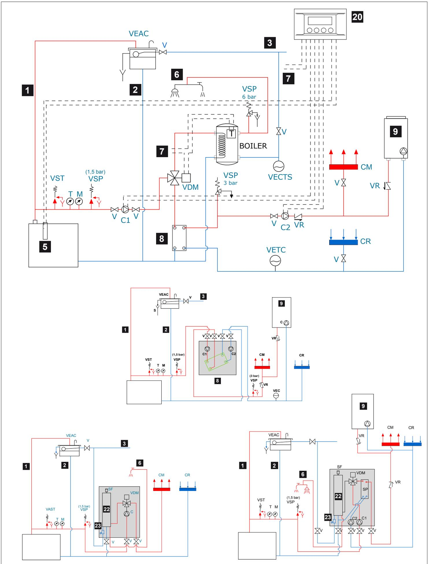
IMPIANTO a vaso CHIUSO / CLOSE chamber / GESCHLOSSENE AUSDEHNUNGSGEFÄSS / INSTALLATION a vase FERME
