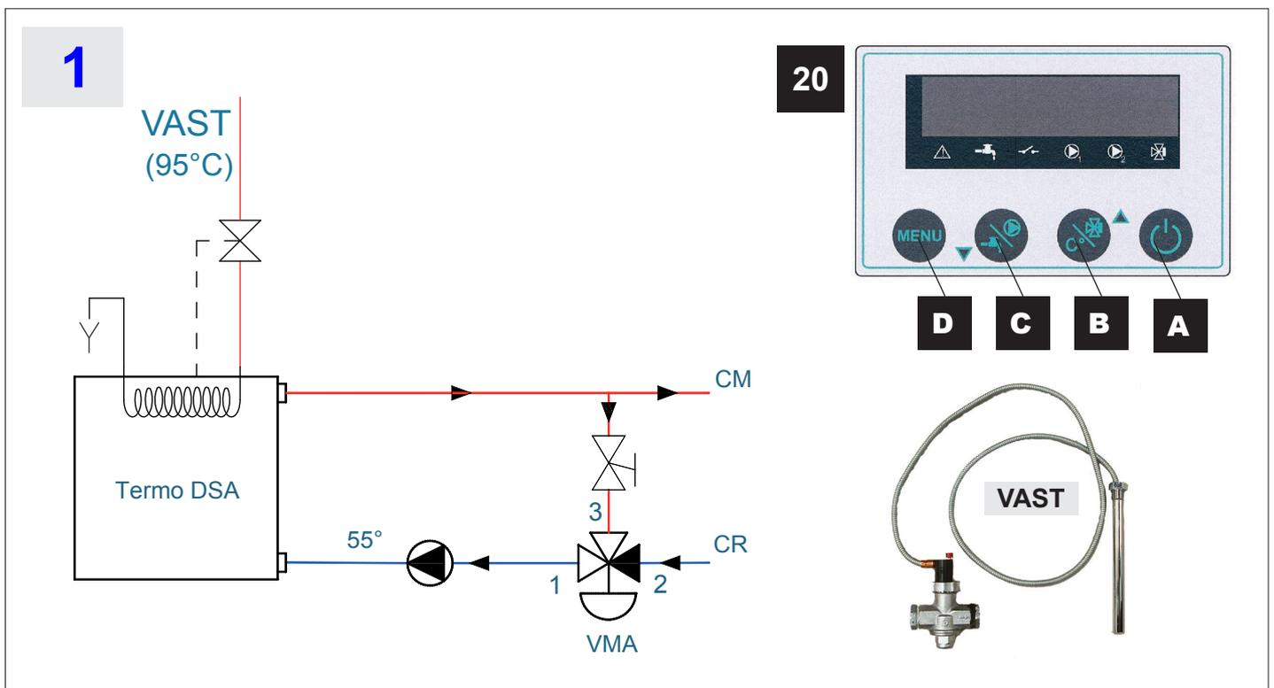
IMPIANTO a vaso APERTO / OPEN chamber / OFFENE AUSDEHNUNGSGEFÄSS / INSTALLATION a vase OUVERT
